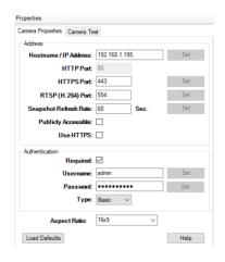
6. The ClareVision camera driver supports the ability for the integrator to choose which camera stream Control4 Navigators will use for streaming video. The driver is defaulted to use the Sub Stream, but can be changed to use the Main or Third stream by navigating to Advanced Properties > Properties. Select the camera stream and click Set.
